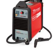
Dual voltage (110V/220V) Inverter plasma cutter. Infinite output adjustment from 5 to 30 amps with high-frequency arc start. 3/8" maximum cutting capacity on steel. Ideal for cutting Aluminum and Ultra-High-Strength Steels.
